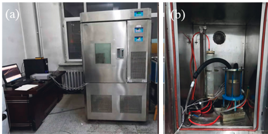
FIGURE 4: Freezing test instrument: (a) free-thaw cycle equipment; (b) water supply system.
