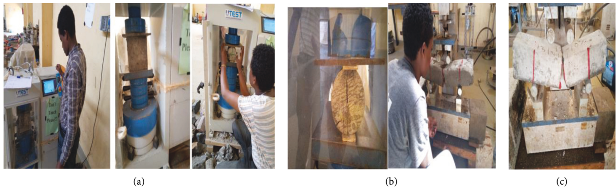
FIGURE 5: (a) Compressive test. (b) Tensile split test. (c) Flexural test.
