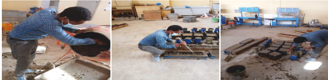
FIGURE 4: Casting concrete test specimens.
