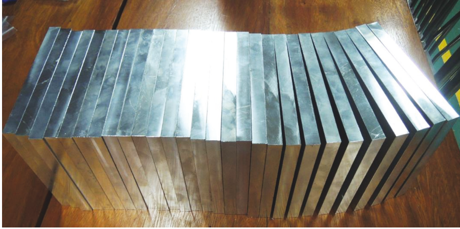
FIGURE 3: AISI 6061 aluminum alloy workpieces for experiments (with permission from [2] (open access)).
