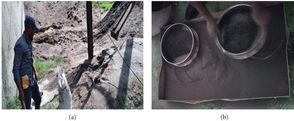
FIGURE 3: (a) Dumping of BA in the open environment, (b) BA sample finer than 150 μm.
