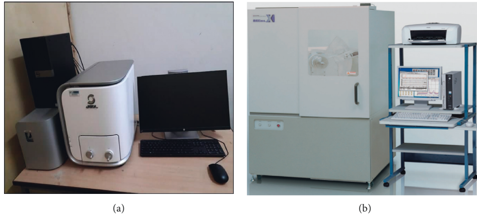
FIGURE 6: (a) JCM-6000 Plus Bench Top SEM JEOL machine. (b) Model XRD-7000 XRD machine.
