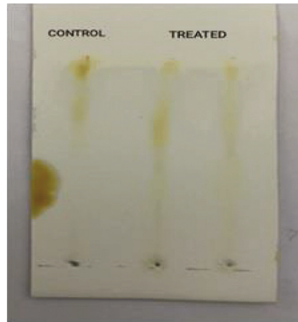
FIGURE 4: TLC analysis for the presence of degraded compound in the treated sample.
