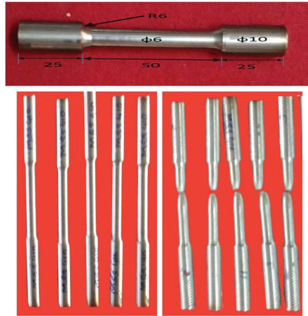
FIGURE 3: Tensile test specimen dimension, before test, and after test specimens.
