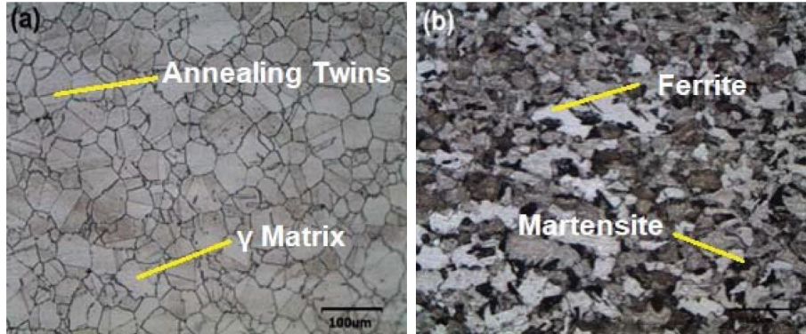
FIGURE 1: Base metal microstructure (a) Inconel 718 and (b) AISI 410.
