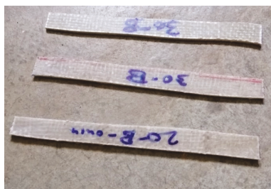
FIGURE 4: Test specimens with the ASTM D 3039 standard.
