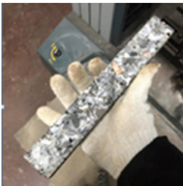
FIGURE 7: Specimen after low-temperature insulation.
