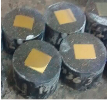
FIGURE 3: Specimen prepared for microscopic examination.
