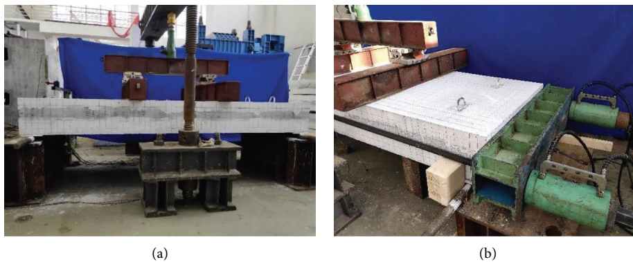
FIGURE 4: Test set-up. (a) Four-point flexural test and (b) axial loading device.
