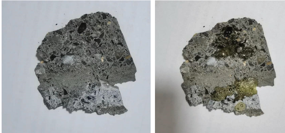
FIGURE 12: Cracking before and after the addition of dilute hydrochloric acid drops.
