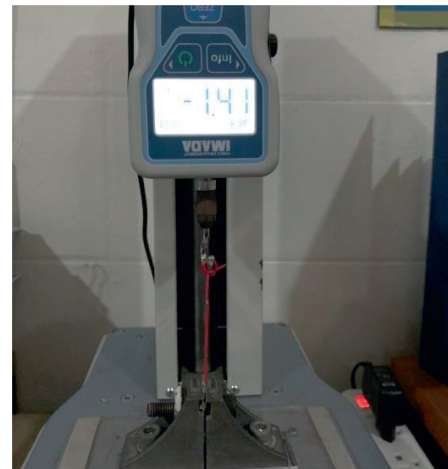
FIGURE 2: A pull testing setup to measure the pull force required to separate a crimped terminal from a wire.
