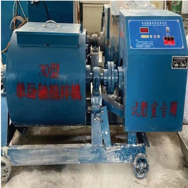
FIGURE 3: Concrete mixer diagram.
