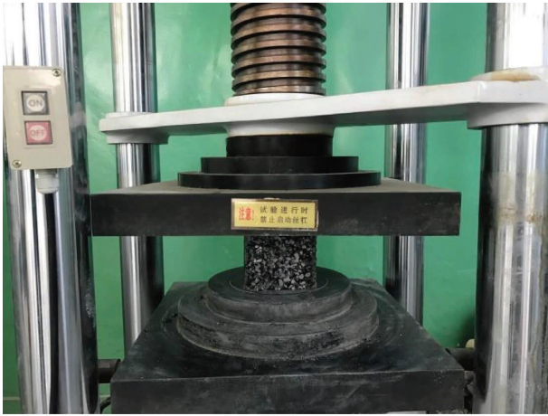
FIGURE 7: experimental device of compressive strength.
