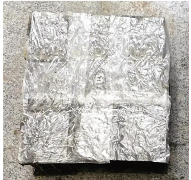
FIGURE 5: Sprinkling maintenance diagram of the cover film of the test piece.
