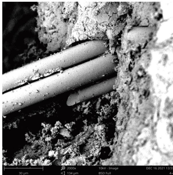
FIGURE 2: Microscopic view of chopped basalt fiber.
