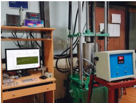
FIGURE 3: Universal tensile testing machine attached with heating chamber and temperature controller (Model: CUTM-50 kN).
