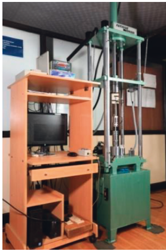
FIGURE 6: Hydraulic universal fatigue and creep testing machine (Model: AVJ-10T).
