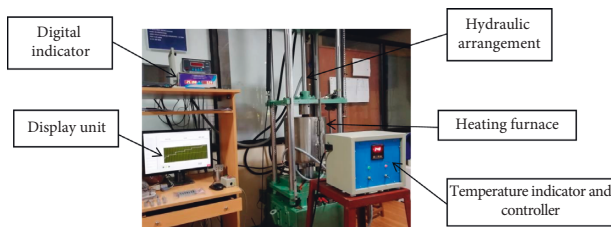
FIGURE 8: Time-dependent creep experimental test equipment.
