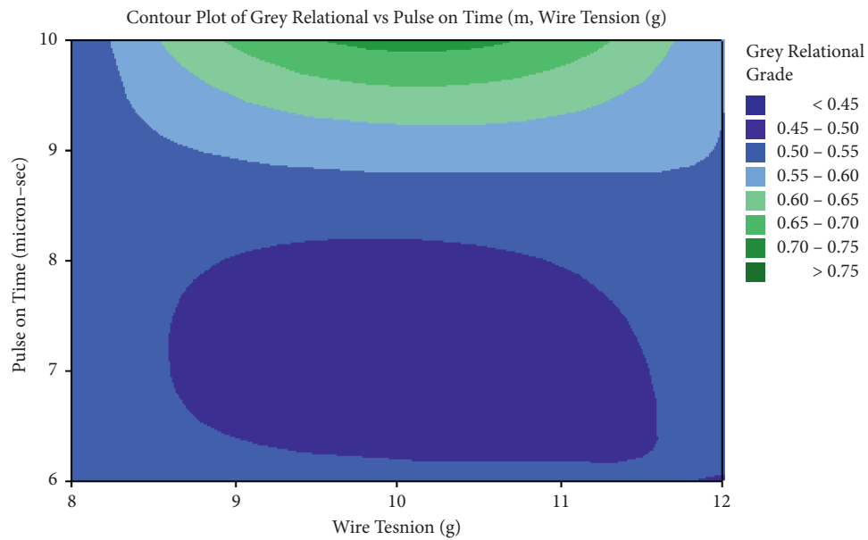
FIGURE 6: Contour plots between pulse on time and GRA.
