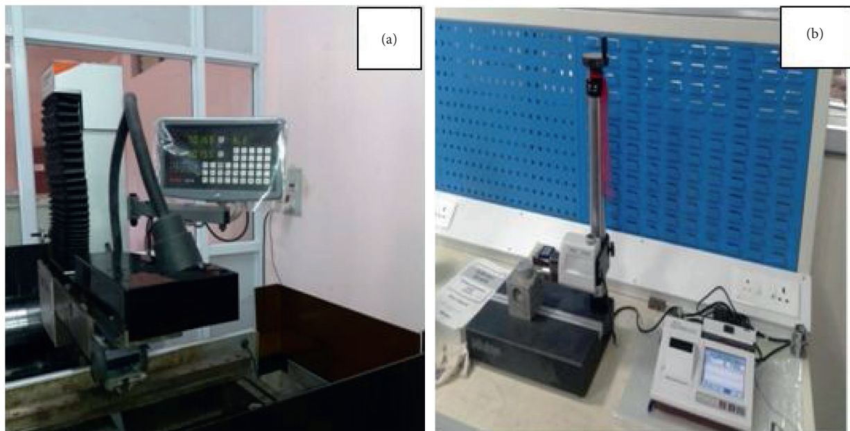
FIGURE 2: (a) Mitsubishi FX series WEDM setup. (b) Surface roughness setup.
