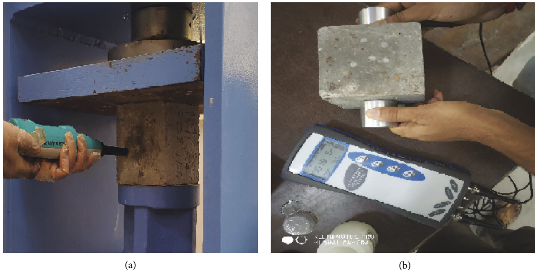
FIGURE 5: Nondestructive tests pics of (a) rebound strength and (b) UPVT.
