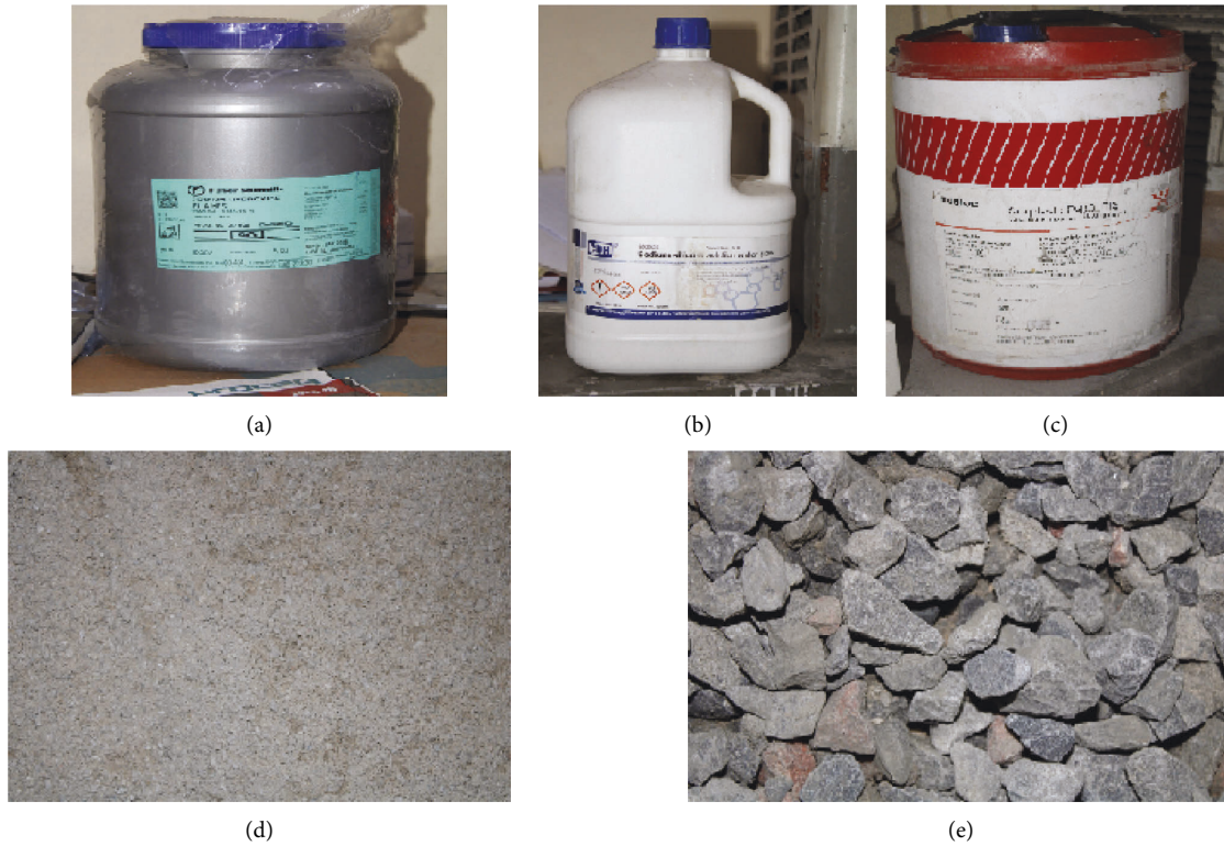
FIGURE 2: Picture of raw materials of the GPC (a) sodium hydroxide flakes, (b) sodium silicate solutions, (c) superplasticizer, (d) stone-dusts, and (e) coarse aggregates.
