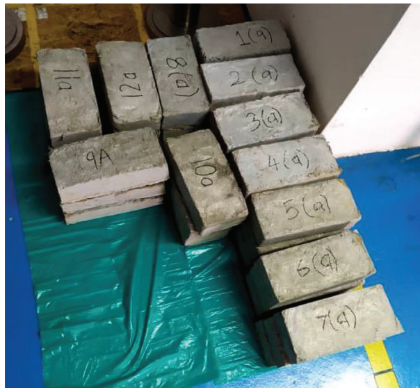
FIGURE 2: Brick samples of different CNS content.
