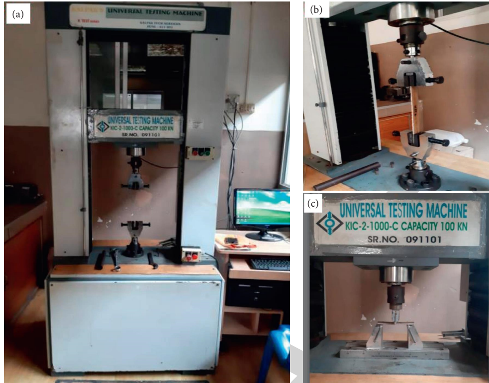
FIGURE 5: (a) Universal testing machine used for the tensile and flexural test (Make: Kalpak Instruments and Controls, Pune, Model: KIC-2-1000-C with the capacity of 100 kN). (b) Tensile test arrangement. (c) Bending test arrangement.
