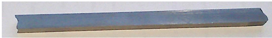
FIGURE 8: The shape of the samples after the first stage of deformation and surface treatment. Workpiece dimensions: thickness is 9 mm, width is 10 mm, and length is 175 mm.
