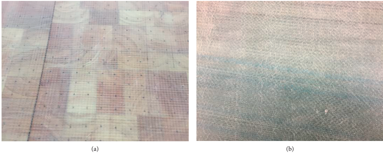
FIGURE 19: (a). Blade surface before sandblasting. (b). Blade surface after sandblasting.
