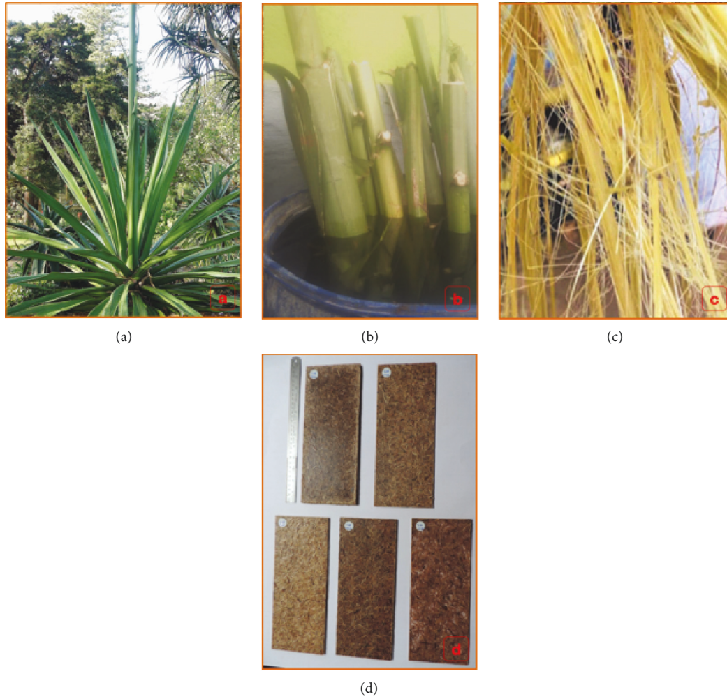
FIGURE 1: Photographs of (a) Furcraea selloa K Koch plant with peduncle; (b) Peduncle under microbial degradation process; (c) Extracted fibers; and (d) FSPF reinforced composite at different weight percentages.
