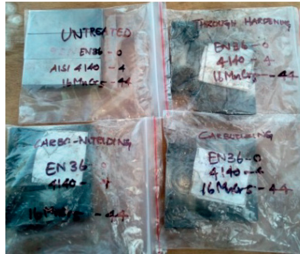
FIGURE 2: Samples from pilot surface treatments including carburizing and through hardening.
