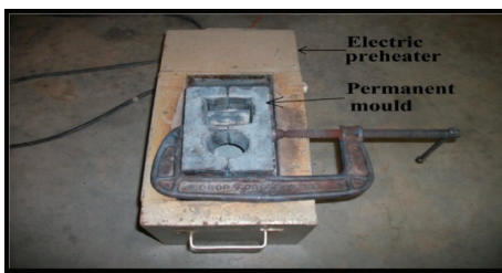
FIGURE 2: Preheater of the permanent mould.
