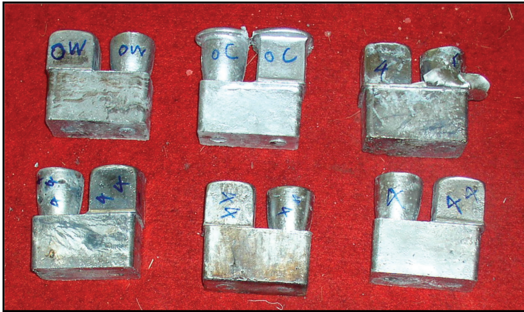
FIGURE 3: Fabricated AA6061/Si 3 N 4 composite castings.
