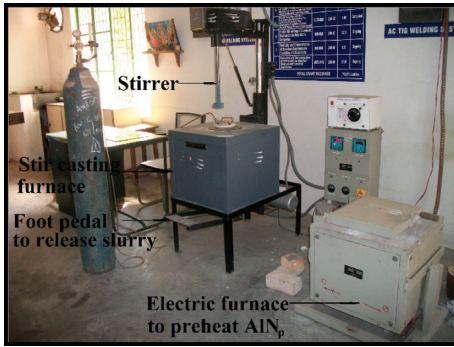
FIGURE 1: Modified electric stir casting furnace with the bottom pouring attachment and the electric furnace used to preheat \text{Si}_3\text{N}_4 .
