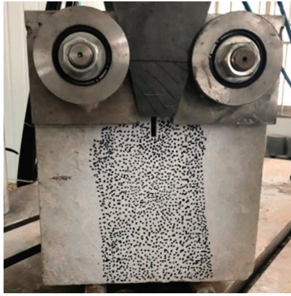
FIGURE 2: Specimen surface with speckle.
