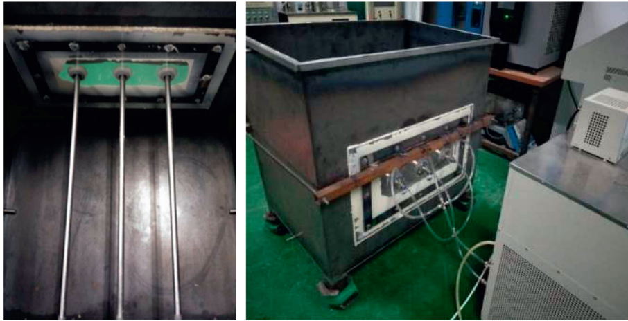
FIGURE 3: Freezing pipes (a) and physical modelling box (b).
