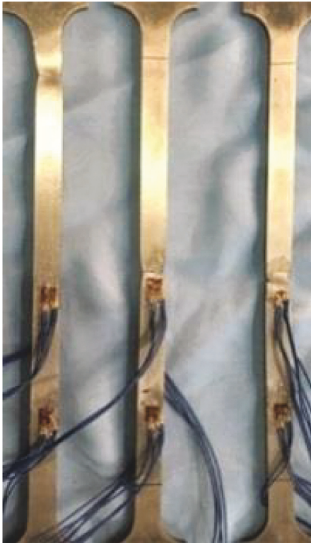
FIGURE 4: Image of a damaged specimen.
