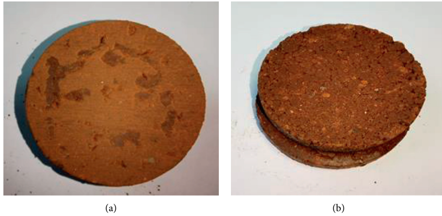
FIGURE 8: Pictures of failed samples. (a) Direct shear test of high plasticity clay-concrete interface. (b) Direct shear test of clay.
