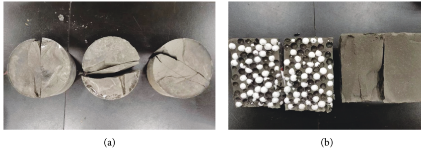
FIGURE 9: Fractured IDT samples. (a) Top view. (b) Side view.
