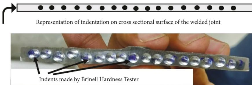
FIGURE 6: Hardness profile of all the samples; the welded zone possesses high hardness.
