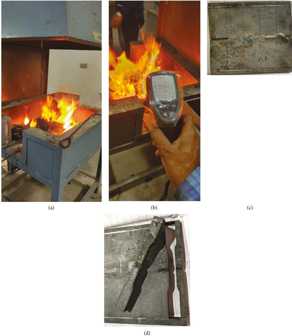
FIGURE 1: Experimental procedure. (a) Welded plates were heated in an open-hearth furnace; (b) temperature values were observed by using a pyrometer; (c) sample preparation for further analysis; (d) a tensile test specimen prepared by using wire-EDM.
