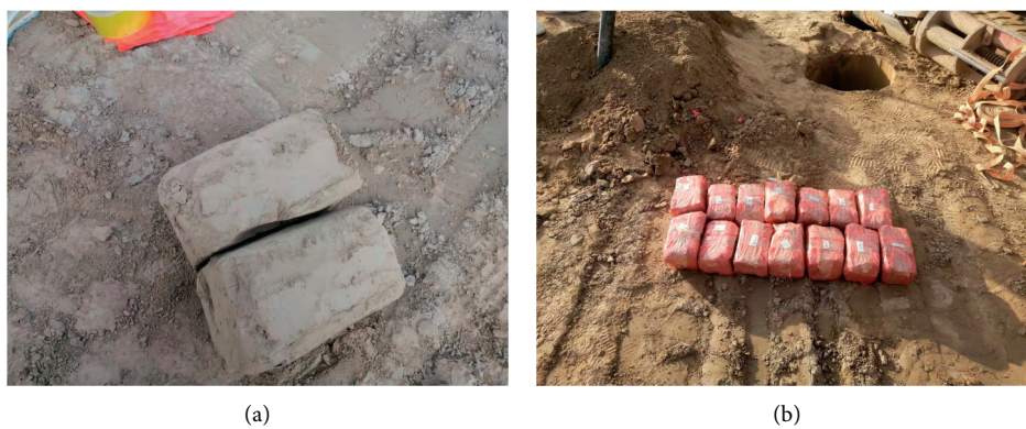
FIGURE 2: Photos of intact loess sampling. (a) Intact soil photos. (b) After intact loess sampling.
