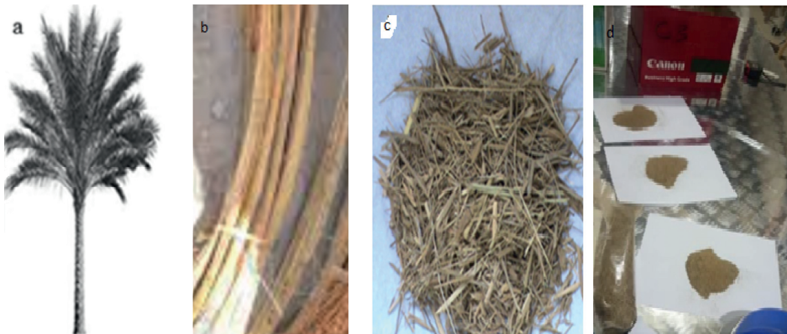
FIGURE 3: Extraction of date palm frond (DPF) fibers.
