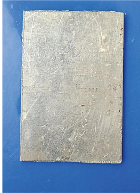
FIGURE 1: AA7010 alloy base metal to be welded.
