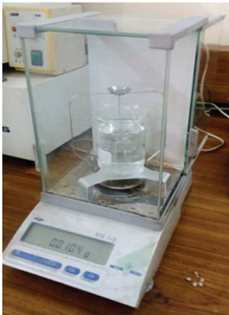
FIGURE 5: Mettler Toledo electronic balance for density measurement.
