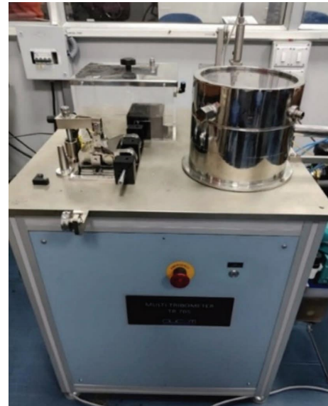
FIGURE 10: Universal tribometer with heat chamber.
