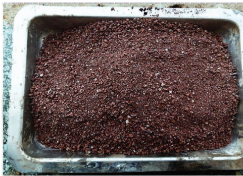
FIGURE 1: Sample of cinder gravel used for the experimental model.
