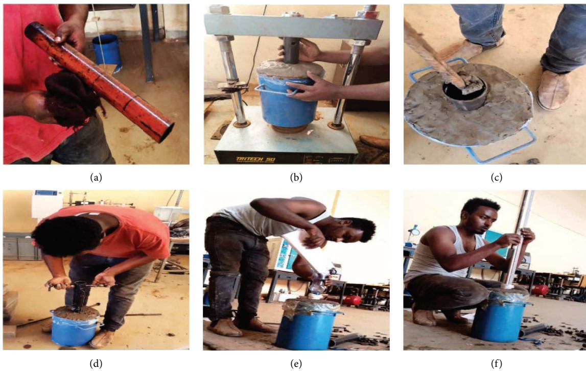
FIGURE 7: (a) Greasing open-ended pipe, (b) inserting open-ended pipe into clay bed, (c) scooping out soil in the pipe, (d) twisting pipe to withdraw, (e) pouring cinder gravel to the prepared hole for cinder gravel column, and (f) compaction of cinder gravel column in to layers.
