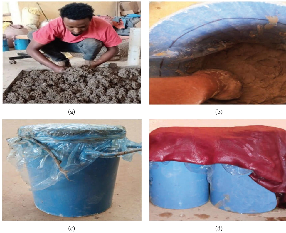
FIGURE 6: Preparation of soft clay bed: (a) mixing air-dried clay soil, (b) placing and controlling during filling test tank with clay paste, (c) tightening with a plastic sheet to keep the moisture content of the clay bed, and (d) covering with a wet cloth for 48 hours.
