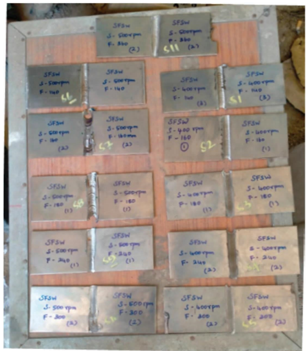
FIGURE 3: Submerged friction stir welded joints at different process parameters.
