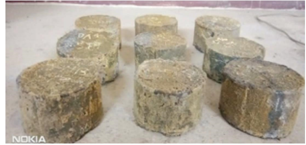
FIGURE 5: Specimens after exposed to acid and sulphate.
