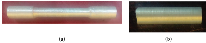
FIGURE 3: (a) Tensile test specimen and (b) wear test specimen.
