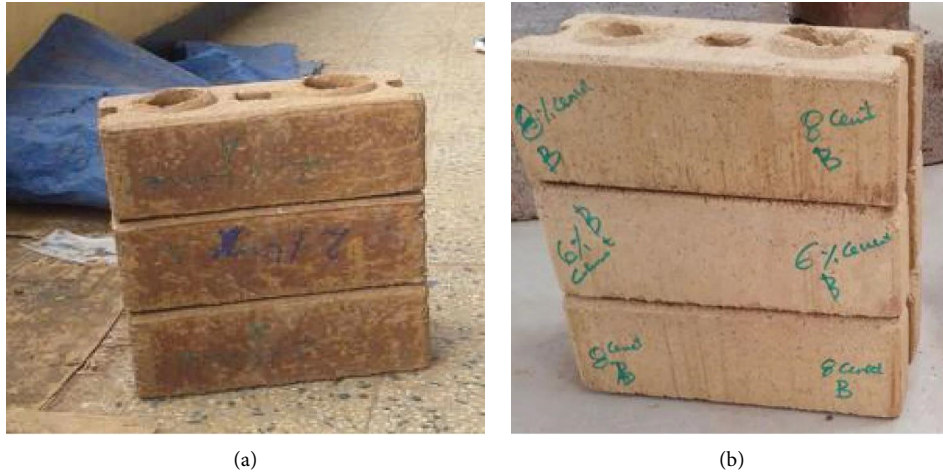
FIGURE 6: (a) Lime-cement-stabilized clay soil block A, (b) cement-stabilized silty sand soil block B.
