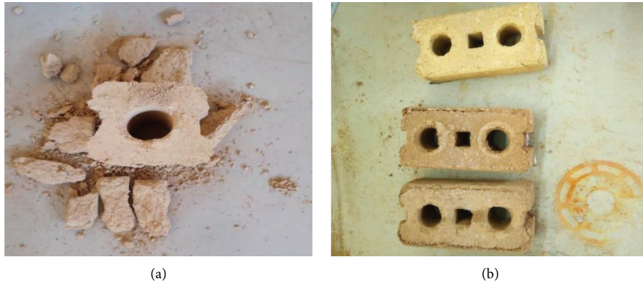
FIGURE 8: (a) Half-length block and (b) full size fracture mode soil block under compression test.
