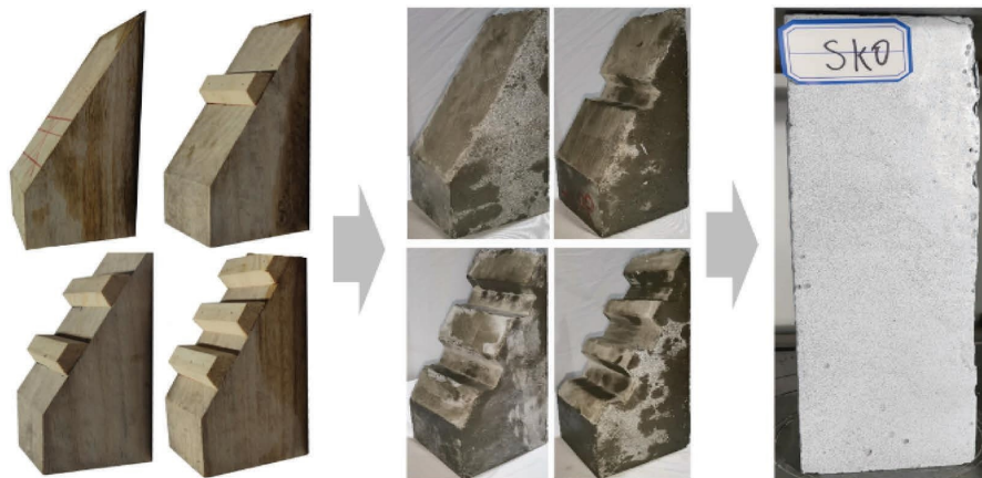
FIGURE 2: The production process of the specimen. (a) Place-holding wooden block cutting. (b) UHPC casting forming. (c) NC casting forming.
