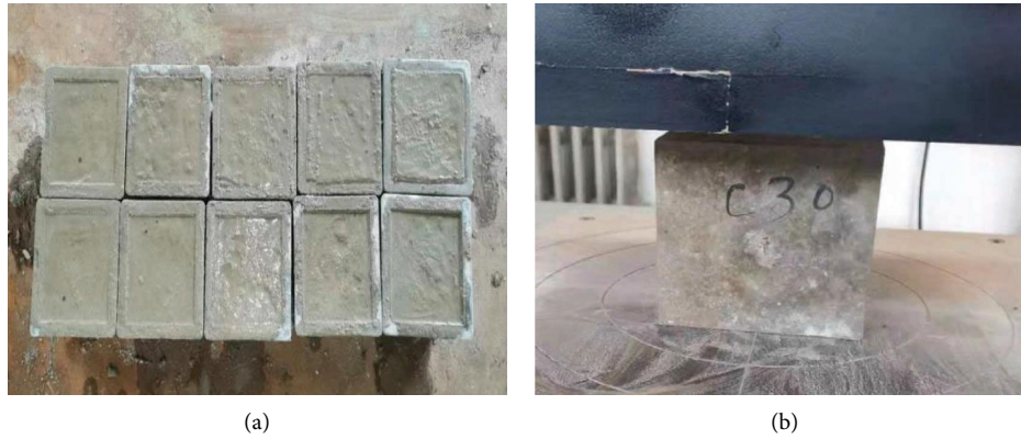
FIGURE 3: Concrete test block configuration diagram: (a) block configuration and (b) compression test.
