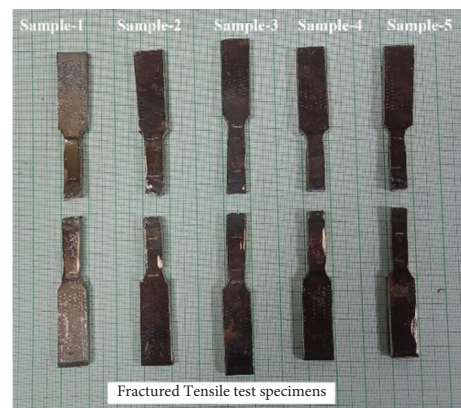
FIGURE 4: Broken tensile test specimens.
