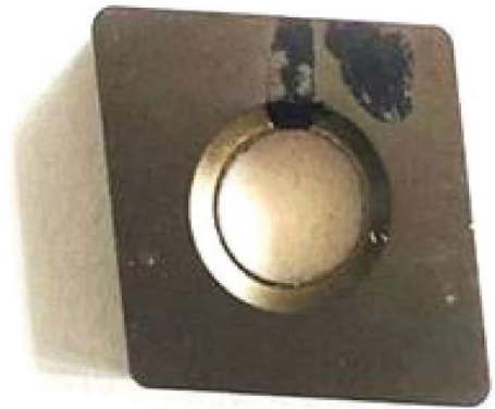
FIGURE 2: CNMA 120408-KR 3215 carbide insert.
