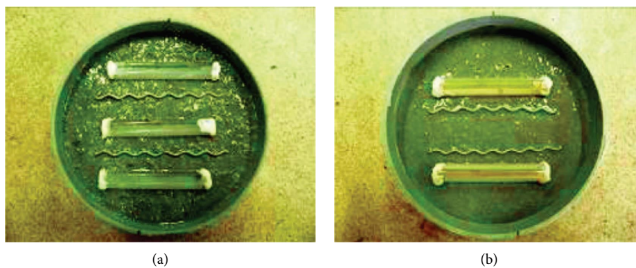
FIGURE 2: Cylinders with the glass tubes which were filled with healing agents: (a) silica sol as carrier and (b) PU as carrier. Reproduced from ref. [27] with permission of Elsevier Ltd., © 2012.
