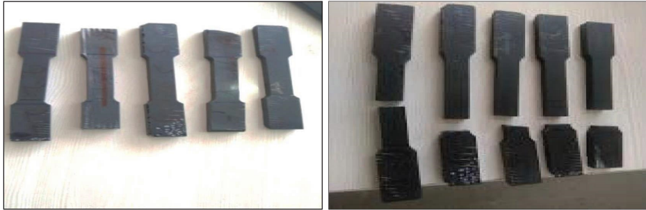
FIGURE 2: Flexural test specimens before and after test.
