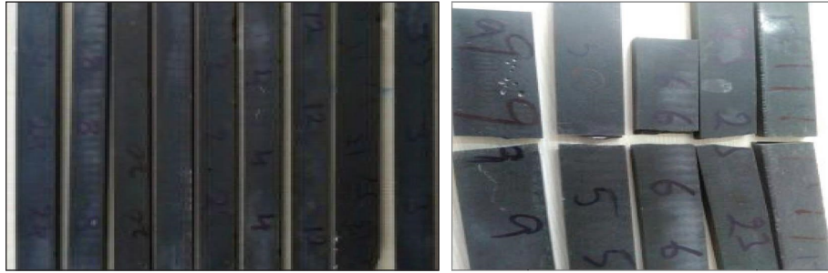
FIGURE 5: Impact test specimens before and after test.
