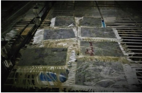
FIGURE 2: Prepared sandwich composite panels in artificial weathering chamber.
