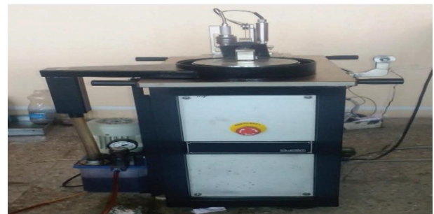
FIGURE 1: Pin-on-disc experimental setup.
