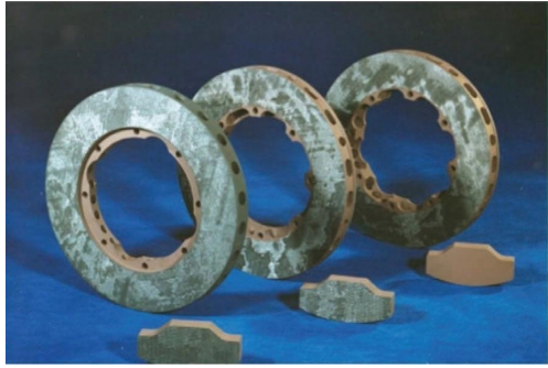
FIGURE 27: Racing car brakes: ventilated discs and pads [165].
