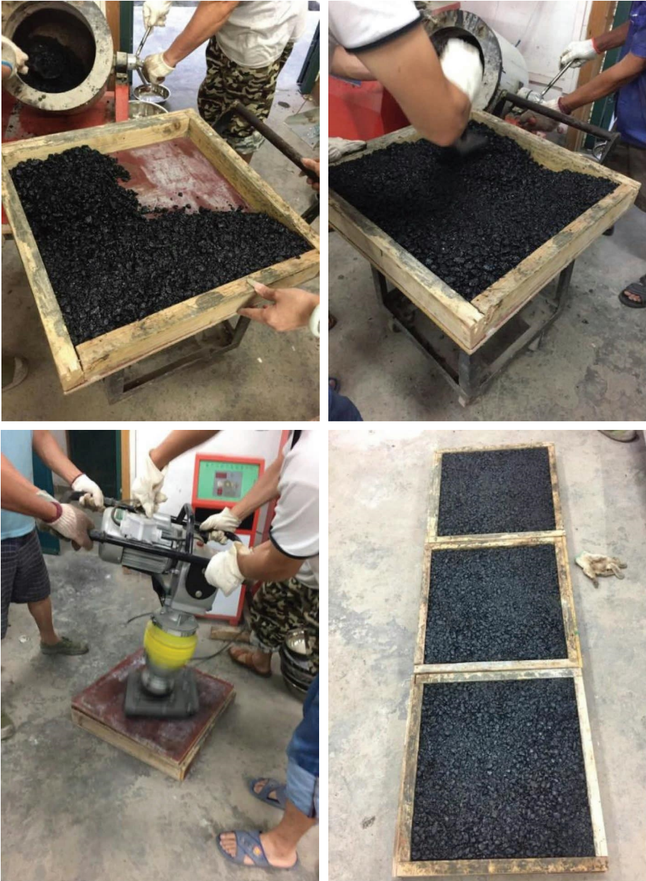
FIGURE 20: Forming process of the hard sandstone AC-13C.
