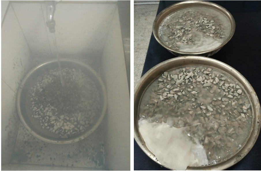
FIGURE 9: Freeze and thaw cycles of the hard sandstone coarse aggregate.
