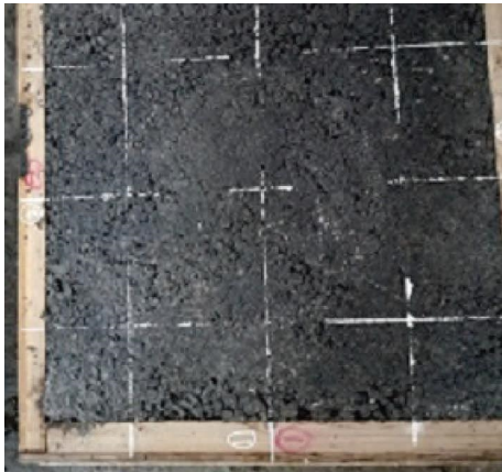
FIGURE 22: Three-wheel polishing test of the hard sandstone AC-13C.
