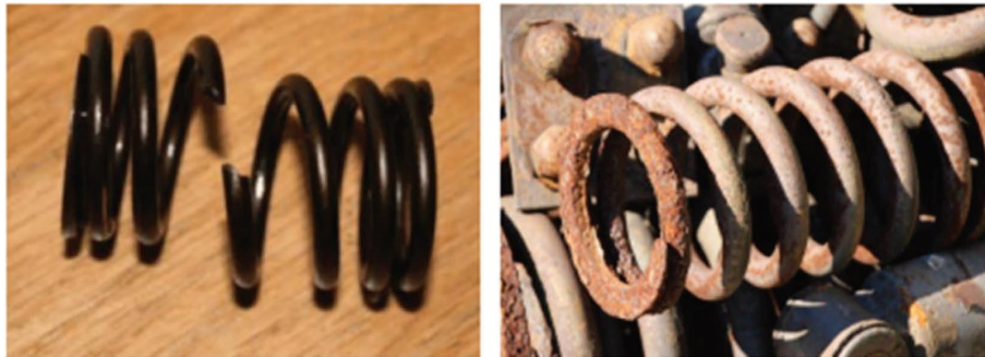
FIGURE 3: Failure of helical vehicle coil springs [6, 7].
