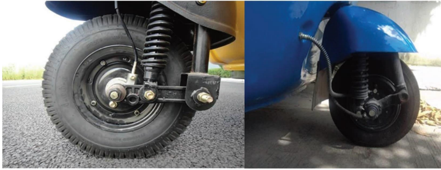
FIGURE 2: Coil spring installed on front suspension of three-wheeler vehicles.
