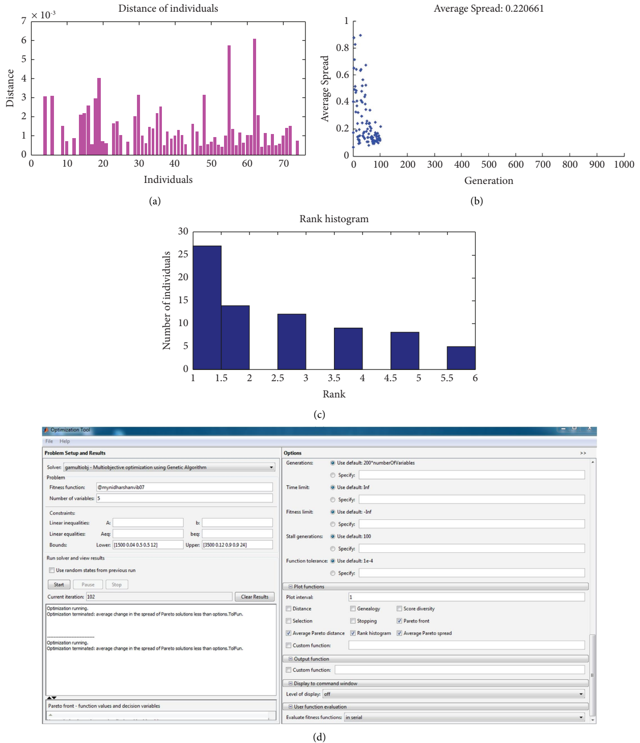
FIGURE 5: Performance of fitness value generation and the best and most consistent variable performances in structured form: (a) distance of individuals, (b) average spread of generations, (c) rank histogram of individuals, and (d) GA optimization tool interface.
